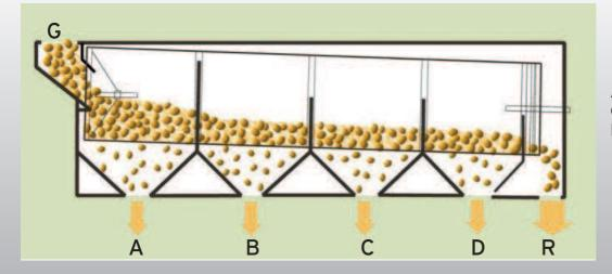
A B C D : Undersized grading G : Input sample R : Malting sample
