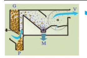
MAROT Aspirators are designed to remove light impurities from the grain and at the same time separate the heavy aspirated material from the light dust.
