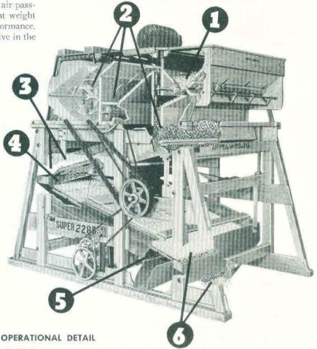
holds up the good commodity and drops the broken, undersized, and poor germinative kernels and other small foreign material to a pan underneath.
