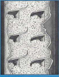
CONTINUOUS MECHANICAL MIXING Lifted rapidly at different speeds, the materials are tossed and tumbled from one spiral to the other. Here is fast, mechanical mixing of materials taking place in the oval housing. This innermixing chamber is an exclusive and fully patented feature of the Blue Streak Twin Spiral Mixer.
