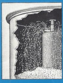
CONTROLLED REMIXING On reaching the top of the oval housing, the materials are tossed in different directions at different speeds and against the sides of the mixer. Falling on the batch, they automatically re-enter the cycle for still further blending. This process is repeated as needed, depending upon the formula or type of feed.
