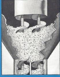
**INSTANT ELEVATION** Large 12 inch spirals instantly deliver the materials up into the inner-mixing chamber and instead of depositing the feed in layers, a constant interchange of materials starts immediately as the first materials reach the cone section. This action continues as the mixer is constantly loaded to the bottom line of the avail housing.
