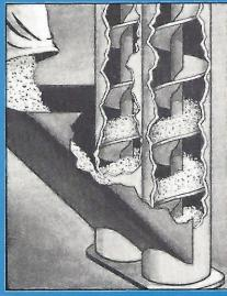
FASTER LOADING A bag is upended into the loading hopper of a Blue Streak and almost immediately its contents are gone, loaded into the mixing chamber by the two large 12 inch spirals — resulting in faster loading, faster mixing.
