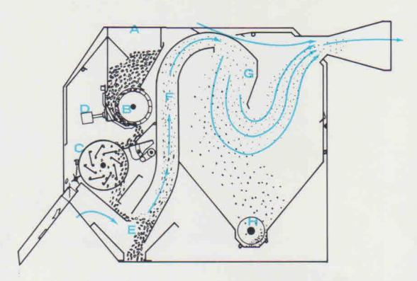
Material enters at inlet (A). Flow at feed roll (B) is regulated by feed control (D). Material is fed at required capacity to Squirrel Cage scalping reel (C) which scalps off sticks, straws, nails and other roughage. Material is then aspirated at (E), where the material leaves the seal gate in an evenly spread stream through which a uniform current of air is drawn. Air liftings or light screenings are carried up air passage (F). This deep passage allows heavier
