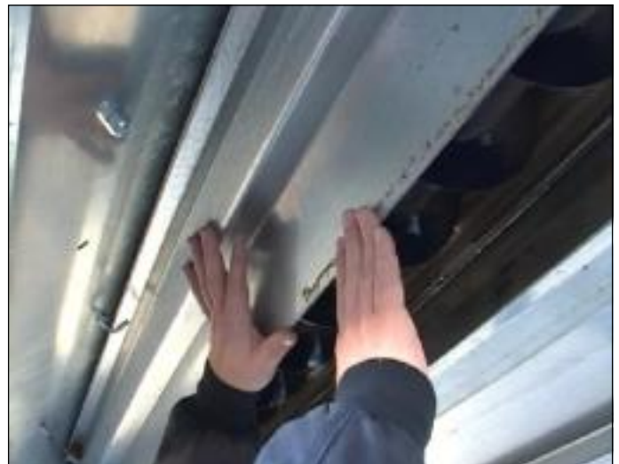
Figure 3.29 - Showing the outer door closed FIRST, then while holding in place, close the inner door.
