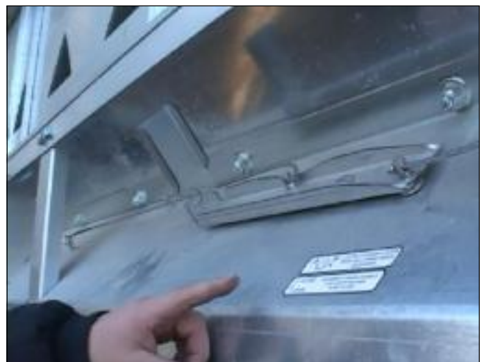
Figure 3.30 - Showing the cleanout doors closed, with the outside handle in LOCKED position. Secure with the steel cable.
