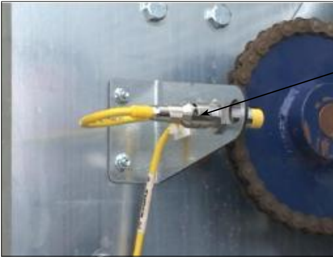
Pancake Switch (Used for Discharge Plugged, Wet Empty, & Dry Full Sensors)
