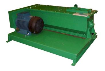
The CW clipper/de-awner is used for pre-treatment of various grain types; the purpose of the de-awning operation is to remove awns from barley kernels, loose husks from wheat, and to clip oat kernels
