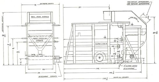
As is true with the Super 29-D the screens can be quickly set up as three tops and one finishing screen by re-arranging special catch-all spouts furnished.
