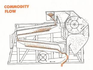
slotted opening which extends across the full width at the bottom of the cleaner.
