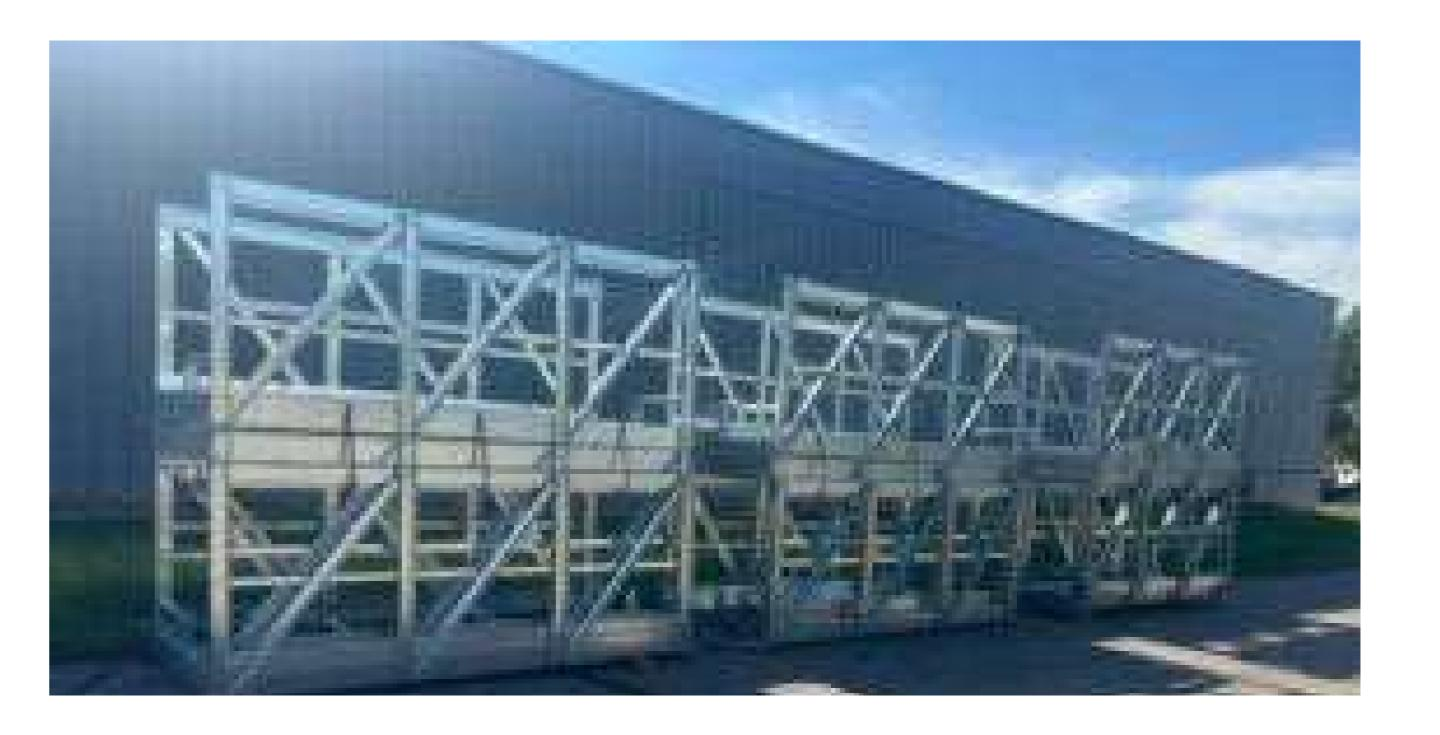
Leg support towers provide stable structural support and ensure safe, reliable operation of the elevator system. **Skywalks** offer safe and convenient access for maintenance and monitoring across the elevator system.
