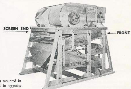
The Super 228-D has two 54" x 60" screens mounted in separate counter balanced shoes and pitched in opposite directions. This counter balancing eliminates excessive vibration and the screen arrangement enables the commodity to travel over the entire width and length of the screens giving better separation at high capacities. Each screen is individually adjusted in pitch.
