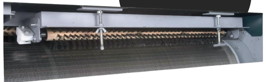
Rotating brush assembly with adjustment bolts and UMHW blocks to prevent damage to the tribar cylinder and clean the slotted holes to prevent plugging. Accessible from a large access door on the side of the units.
